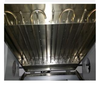
Topside convection heaters ensure the best soldering results even on the most challenging assemblies. Top heaters can be installed directly over the bottom preheat for additional preheating and/or directly over the solder pot for continuous process heat.
