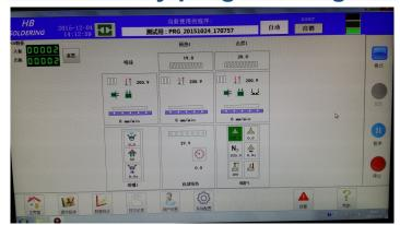
Offline programming software is included and can be used either with Gerber or JPG's, inputting the x and y coordinates. There is no need to interrupt production to make new programs.
