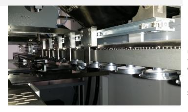
Unique heavy duty board clamping system ensures stability of PCB during soldering and fluxing.
