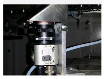
Live viewing of the soldering can assist in the process setup and continuous monitoring throughout the process. Both video and still images can be acquired from the software for archiving.
