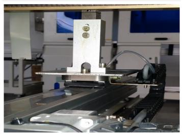
With a 130-micron orifice controlled by a closed loop servomotor, accurate flux deposition is guaranteed.
